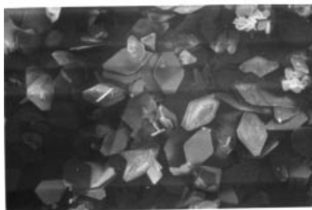
Figure 1. Morphology of as-synthesized samples. (a) K, Na-FER zeolite, \times 1000 , (b) siliceous FER zeolite, \times 70 .
